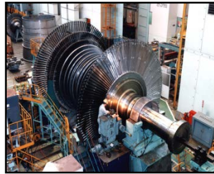
52inch long turbine blade
