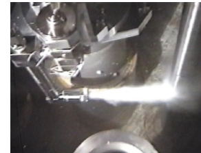
Water Jet Peening
